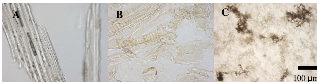
Fig. 3 A. grandis wood particles before any pretreatment (A), after pretreatment with 8 ml and with 25 ml of 85% phosphoric acid for 1 hr at 50°C in a hot water bath (B) and (C), respectively. The samples shown in B to C correspond to the experiments on glucose production presented in Fig. 1
